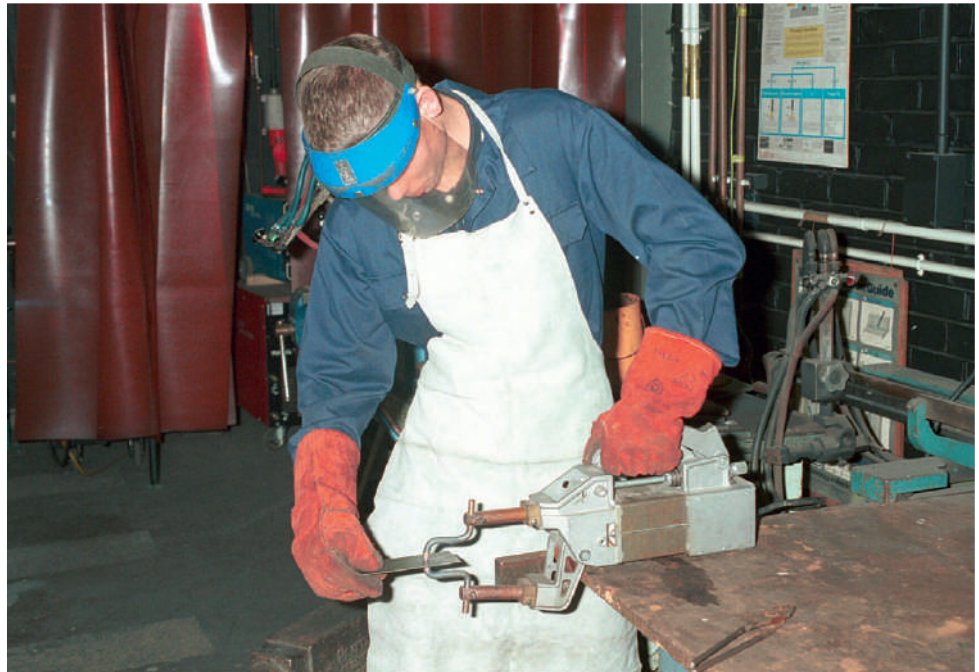
Figure 1.39 Protective clothing for spot welding
